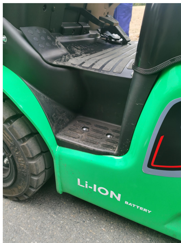
Picture 14 Access step and compartment floor
