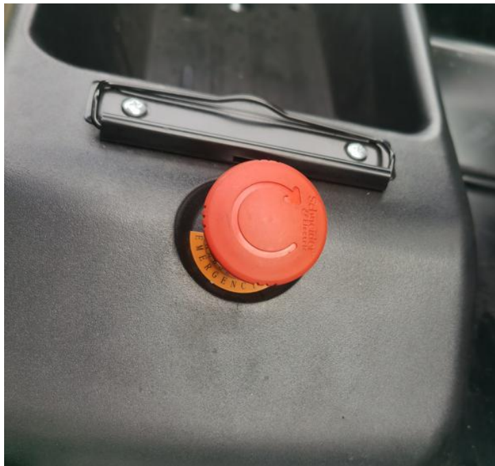
Picture 8 Emergency stop
