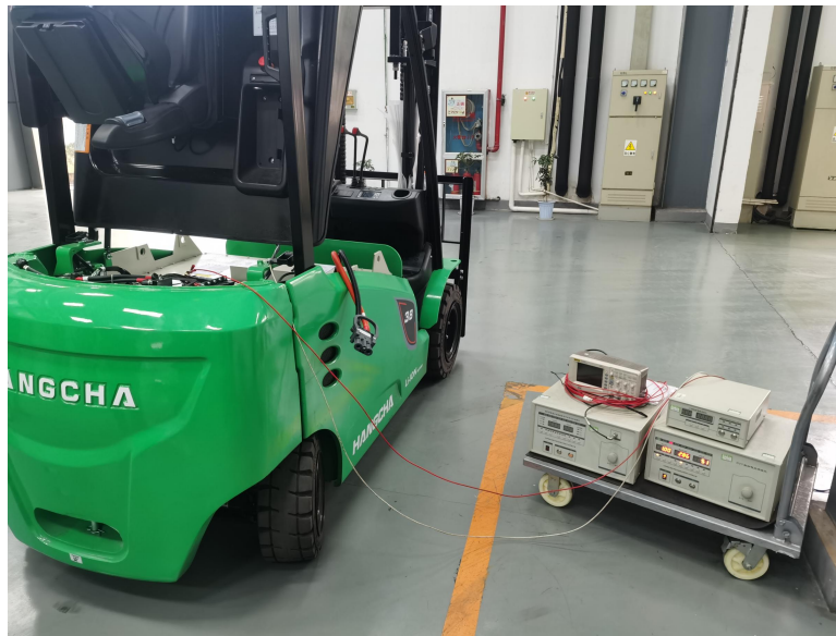
Picture 33~34 Dielectric test and insulation tests
