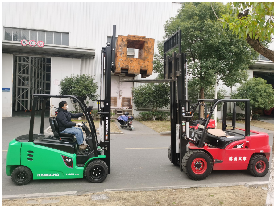
Picture 28 Structural test (1.33Q)
