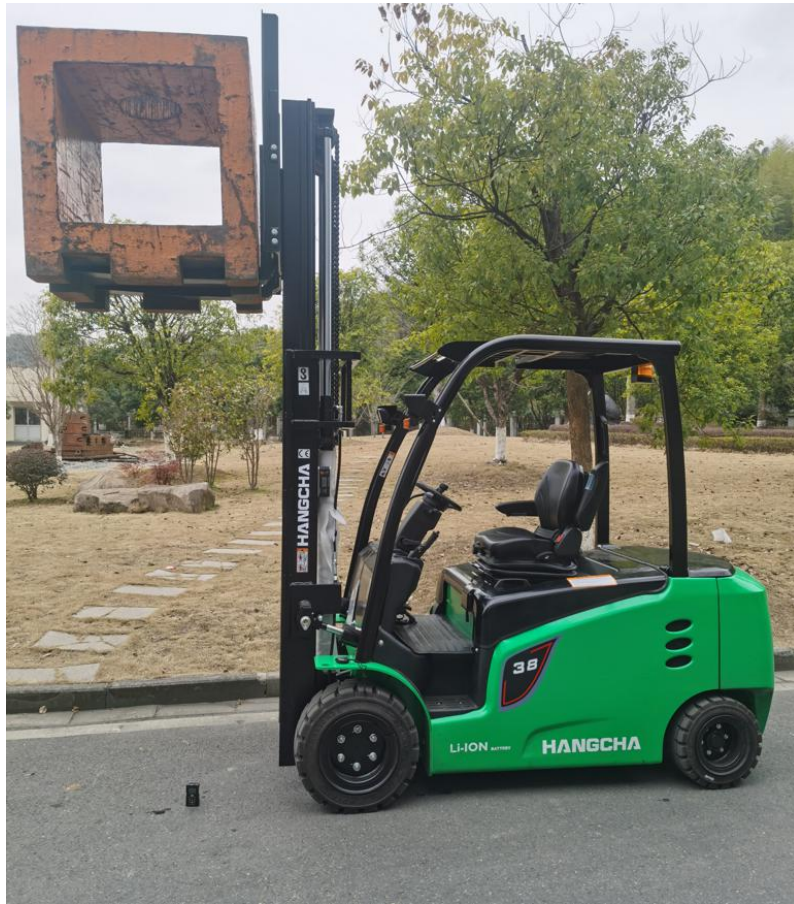
Picture 27 Hydraulic lifting and tilting system test
