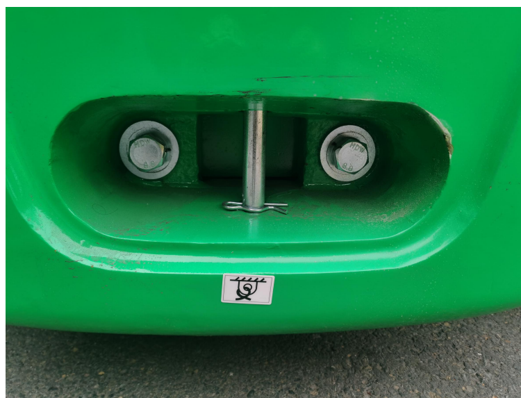
Picture 18 Tie down point
